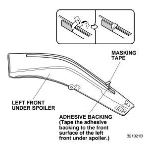
10. Using one alcohol swab, thoroughly clean the front bumper where the left front under spoiler will attach.
